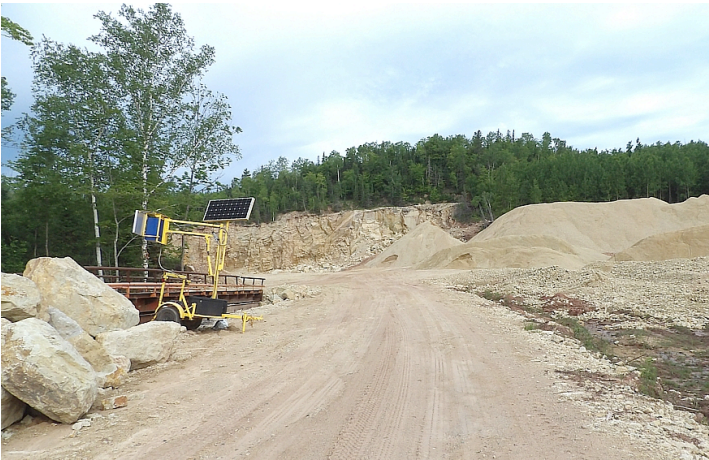
This photo, taken near the quarry entrance, shows large piles of crushed rock, with part of a 50' high by 300' long highwall behind them. The geology of Limestone Mountain is quite complex, and the highwall shows rock layers in a lot of different orientations.
